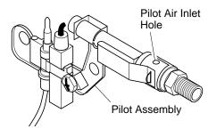
Figure 30 - Pilot Inlet Air Hole
